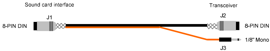
Figure 5 – Orion interface cable wiring diagram
