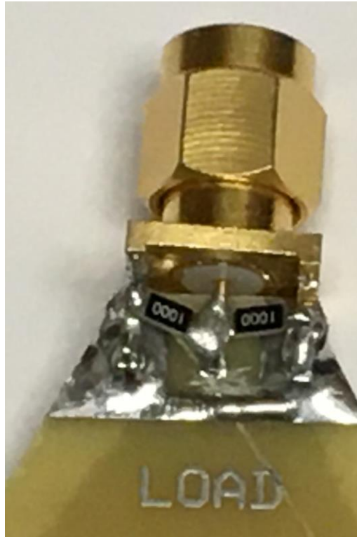
Figure-2, Installation of the two resistors
