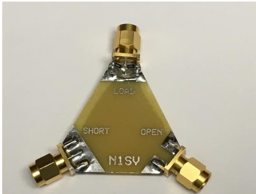
Figure-1, homemade VNA calibration kit
