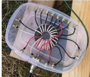
**Figure-3, Impedance Transformer**
