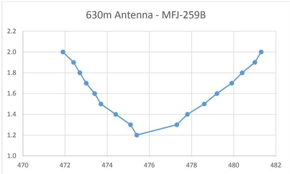
**Figure-7, 630m Antenna SWR using MFJ-259B**
