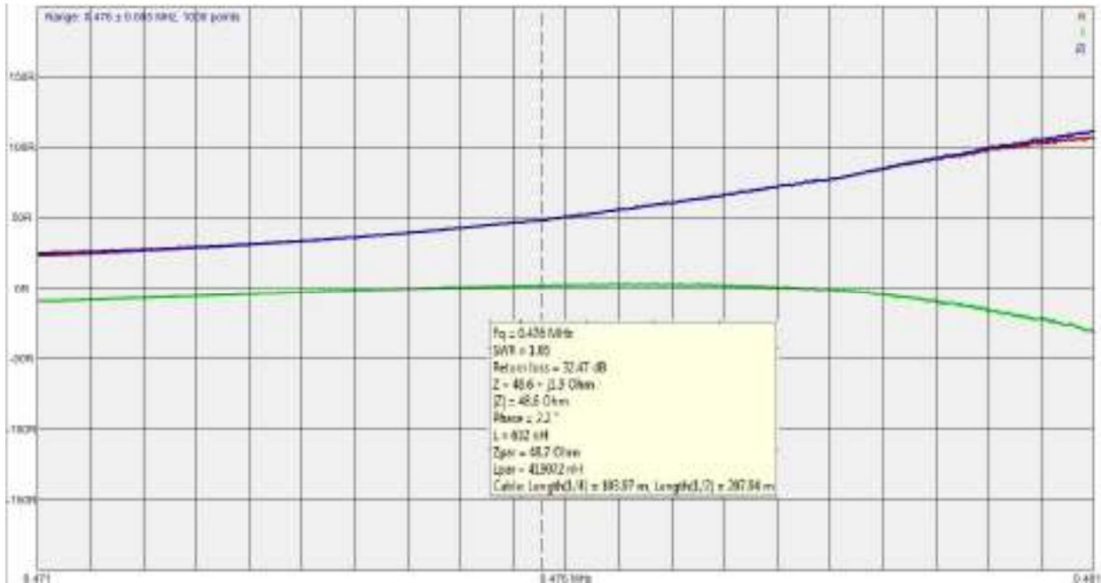
**Figure-9, 630m Antenna RXZ using RigExpert AA-54**
