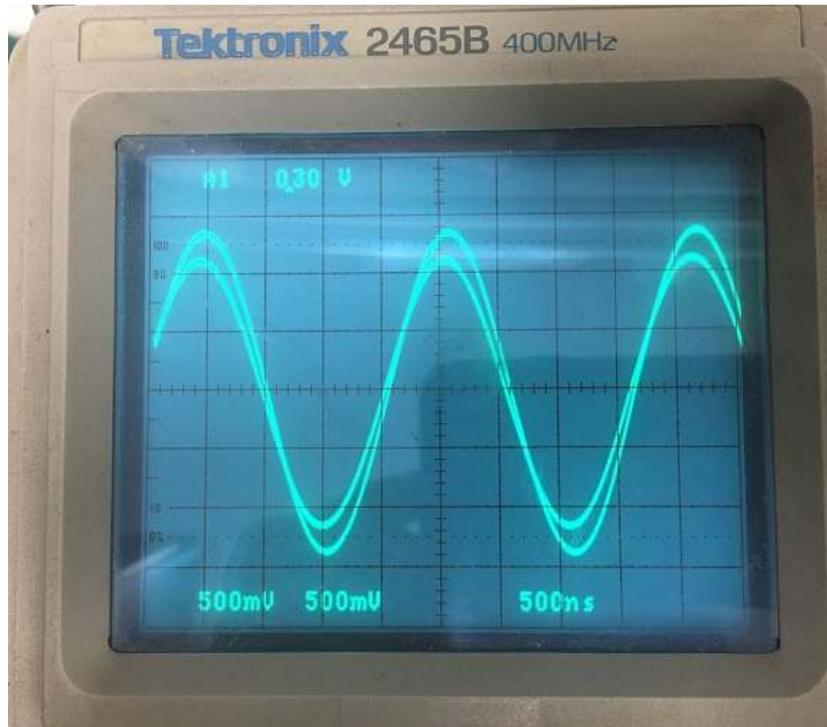
Figure-10, Scopematch waveform of my 630m antenna @ 475.7 KHz
