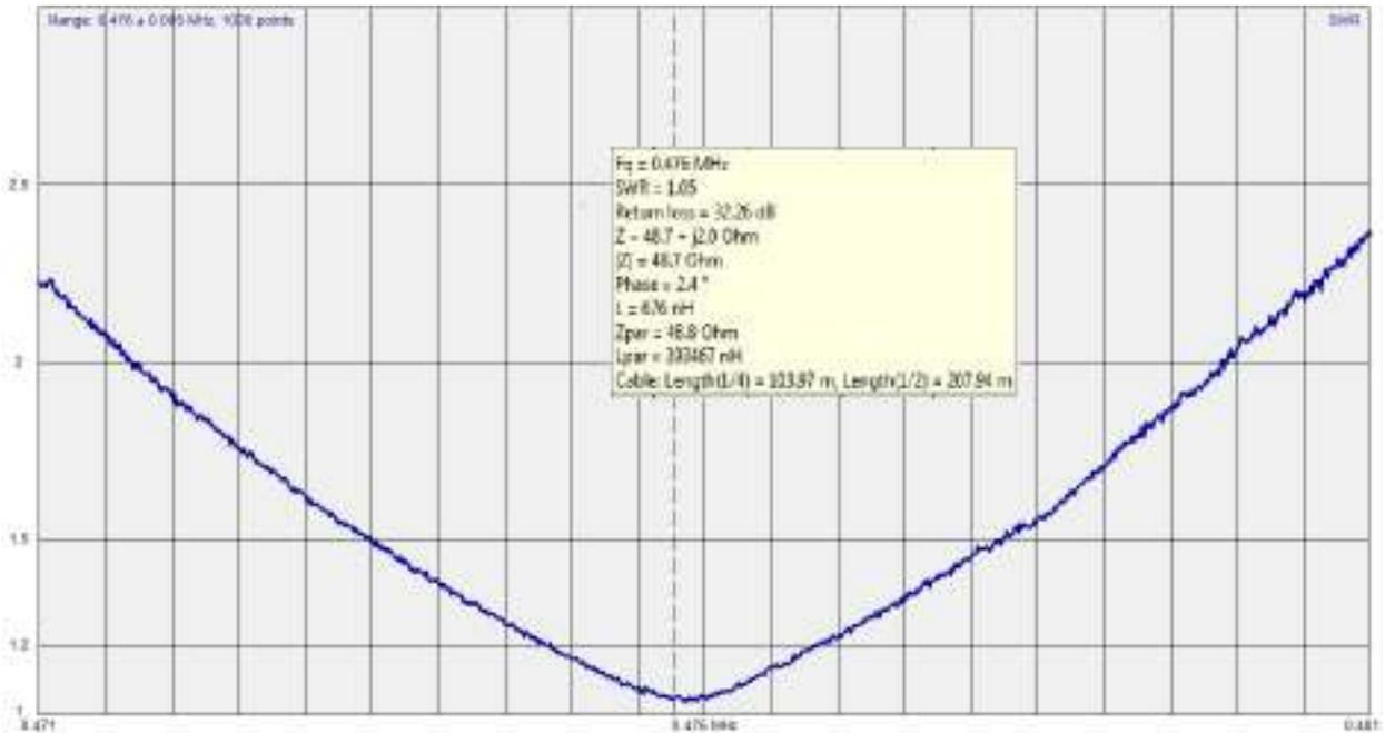
**Figure-8, 630m Antenna SWR using RigExpert AA-54**
